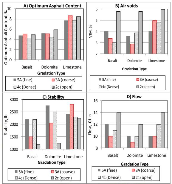
Figure 3 Effect of aggregate type and gradation on mix properties
