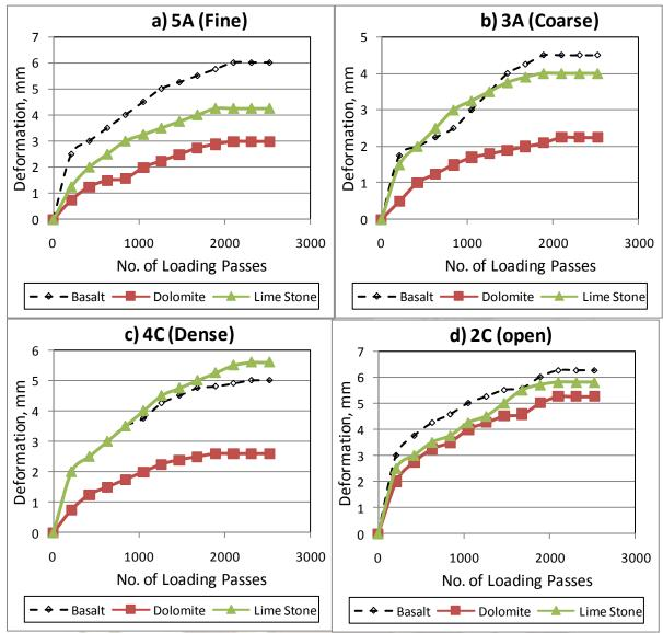
Figure 5 Effect of Aggregate source on Rutting
