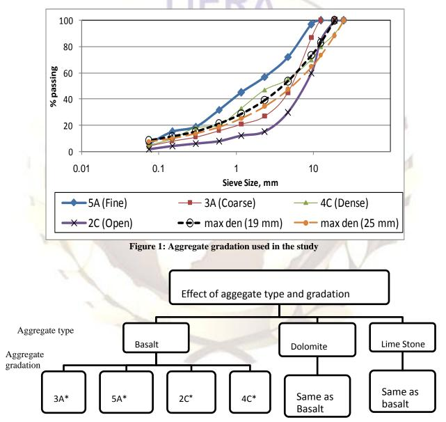
\*: Gradation Type according to Egyptian Specification Figure 2: Summary of Experimental Design
