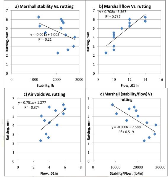
Figure 6 Relation between Marshall mix parameters and rutting
