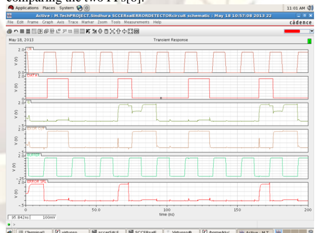
Fig 4.4: Simulation result for Error Detection circuit using SAL technique.
