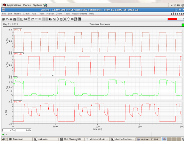
Fig 4.2: Simulation result for MHLFF using SAL technique.
