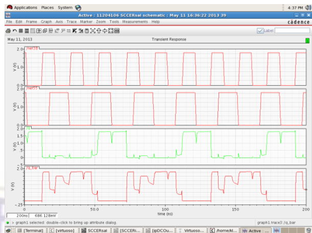
Fig 4.3: Simulation result for SCCER using SAL technique.
