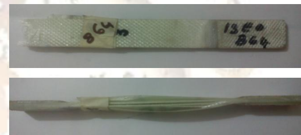
Figure 4.4.2(a): Test specimens of 3mm thickness before and after the tensile test
