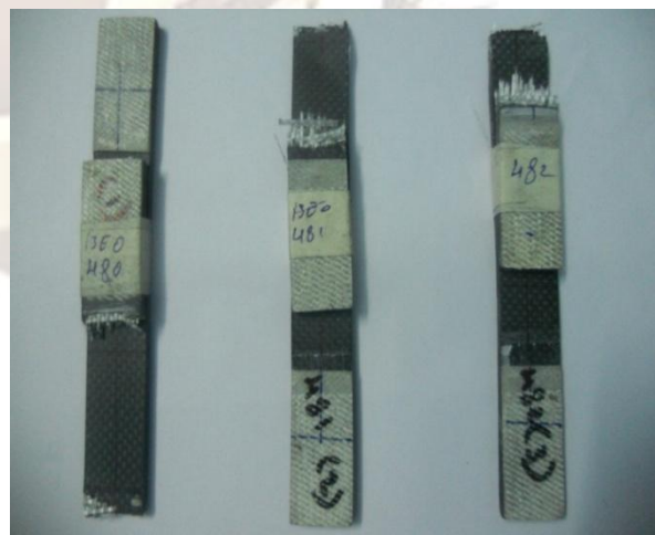
Figure 4.3: Test specimens of 4mm thickness before and after tensile test
