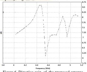
Figure 6. Directive gain of the proposed antenna
