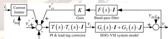
Fig. 9. Control diagram of the SEIG-VSI system with improved DVC.
