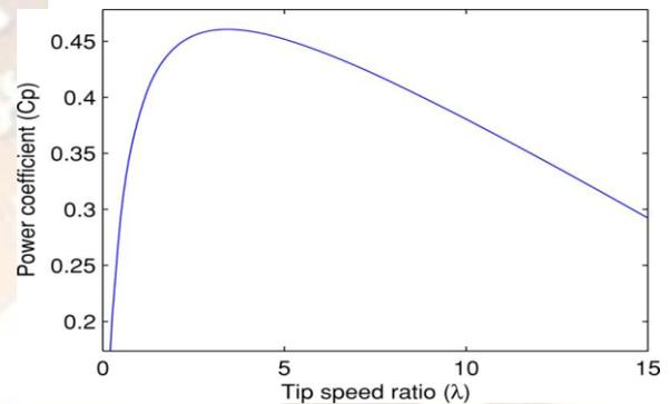
Fig. 2. Typical  $C_p$  versus  $\lambda$  curve.
