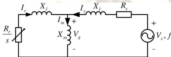
Fig. 3. Single-phase equivalent circuit of the SEIG-VSI system
