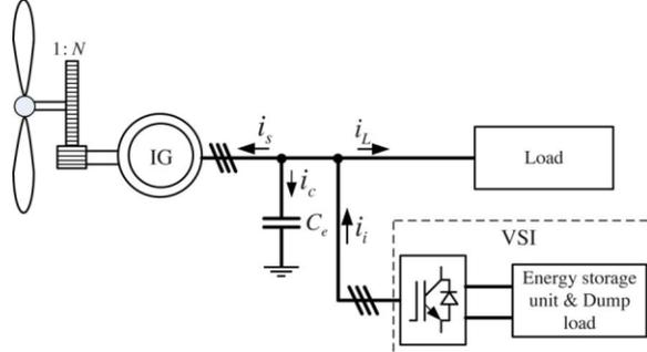
Fig. 1. Block diagram of the SEIG-VSI system.
