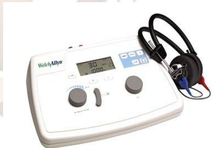
Figure 3. The Welch-Allyn AM 182 Manual Audiometer (above) is one of the most popular on the market, but contains several flaws.
