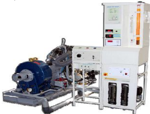
Fig. 1 3-Cylinder MPFI water cooled computerized SI engine
