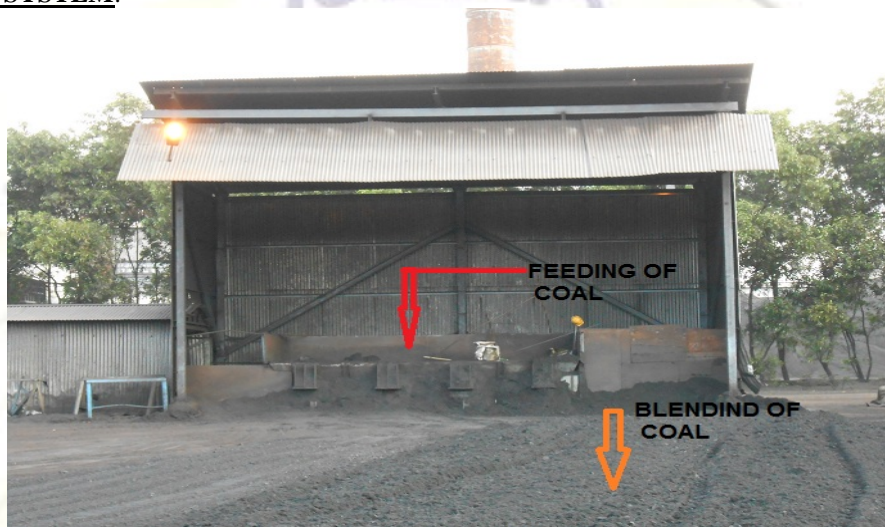
Fig:9 feeding & blending of coal
