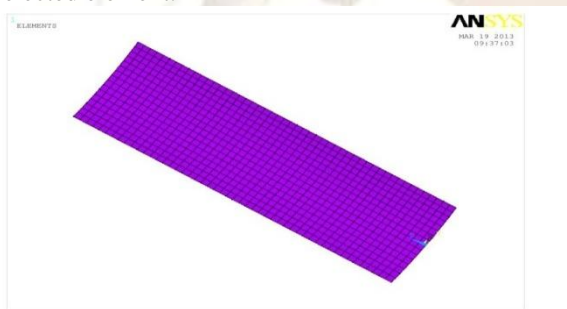
Fig: 4.3 Meshing of Optimize Blade design
