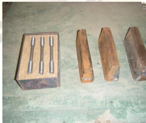
Figure 12. Specimens for tensile test and Microstructure
