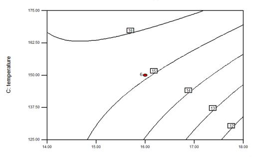
A: moisture Figure 5: Contour plot showing effect of Temperature and Moisture on WSI
