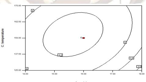
A: moisture Figure 4: Contour plot showing effect of Screw speed and Temperature on WAI
