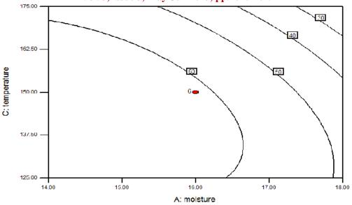
Figure 2: Contour plot showing effect of Temperature and moisture on SME
