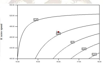
A: moisture Figure 3: Contour plot showing effect of Screw speed and Temperature on Density
