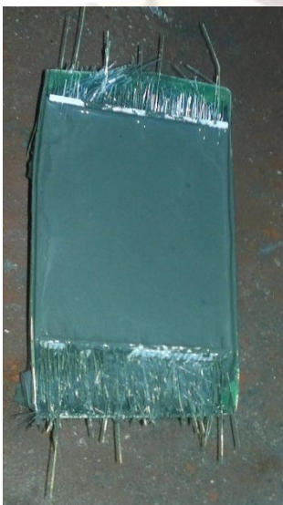
Figures 2.3 and 2.4 showing the setup of the block before concrete being poured in and after.
