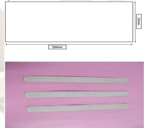
**Test Coupons Preparation:** After cutting the material it's should be cleaned then gripping surface to attach the coupons as per the ASTM E 466-01 standard. If the gripping material should be rough in nature so will place the 1mm aluminum plate on both sites. By using the araldite nature so will place the 1mm aluminum plate on both sites. By using the araldite resin and hardener to paste the plates. Then it's should de
