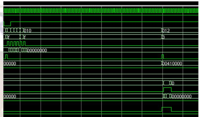
Fig. 4. Waveform of read/write on XDC-CFG interface and command on XDC-Slave-TX interface
