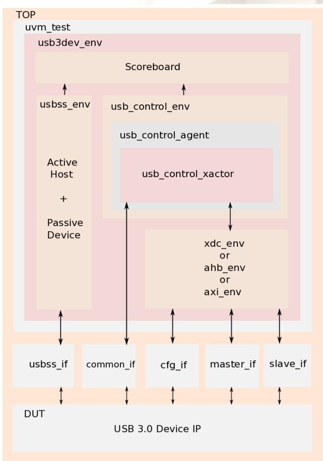
Fig. 2. Verification Architecture using UVM
