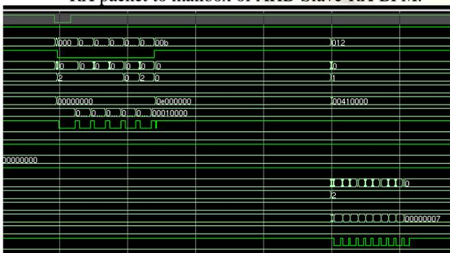
Fig. 6. Waveform of read/write on AHB-CFG interface and command on AHB-Slave-TX interface
