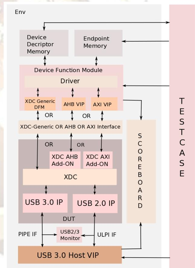
Fig. 1. USB 3.0 Device IP Verification
