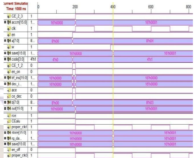
Fig.10: Simulated result of SUB (4-3) operation
