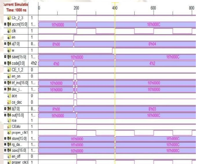
Fig.11: Simulated result of MUL (4*3) operation
