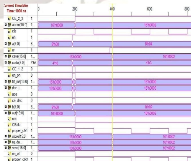
Fig.12: Simulated result of DIV (4/2) operation
