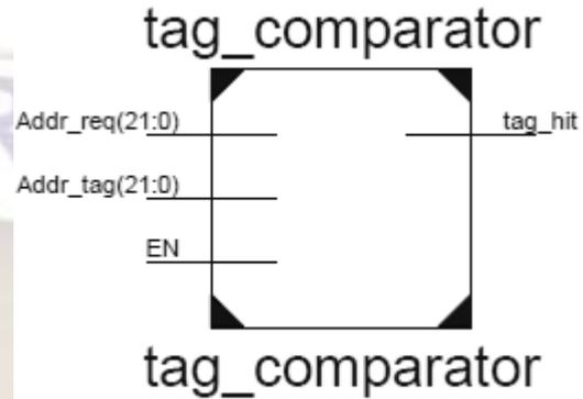
Figure 4: 22-bit cache tag comparator
