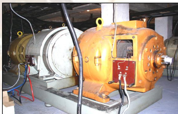
Figure.10. Synchronous generator with prime mover DC motor
