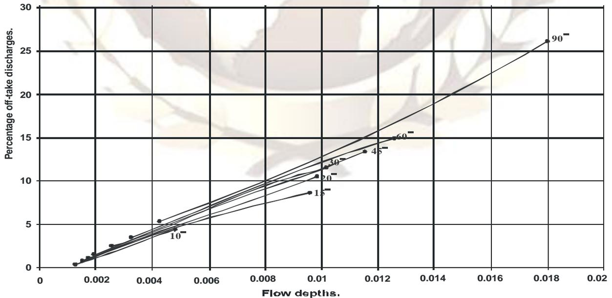
**Fig.3: Variation of flow depths with off-take discharges at convex channel bifurcation.**
