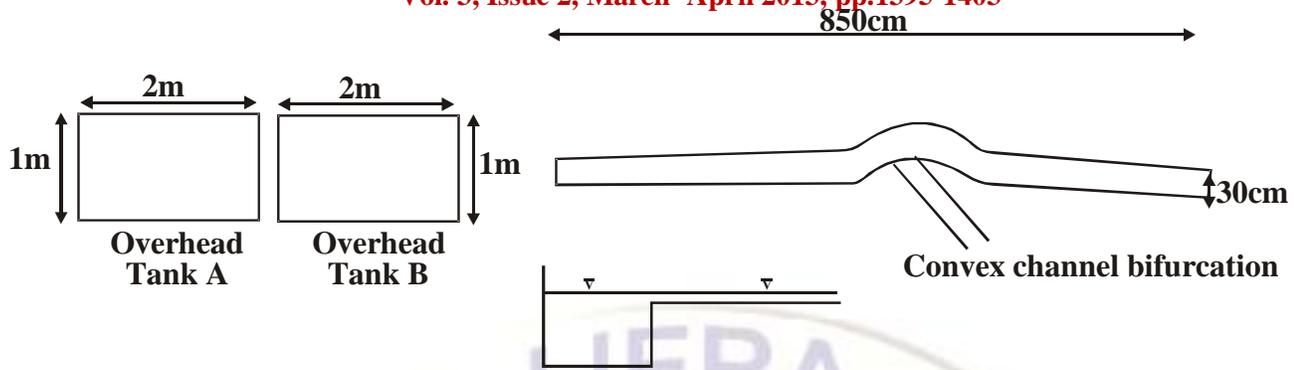
Fig. 1: Plan views of main channel, off-take channel and cross- section.
