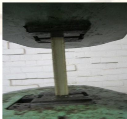
Fig. 2: Position of Bamboo strip in UTM
