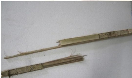
Fig.10: Split Failure of Bamboo Strip
