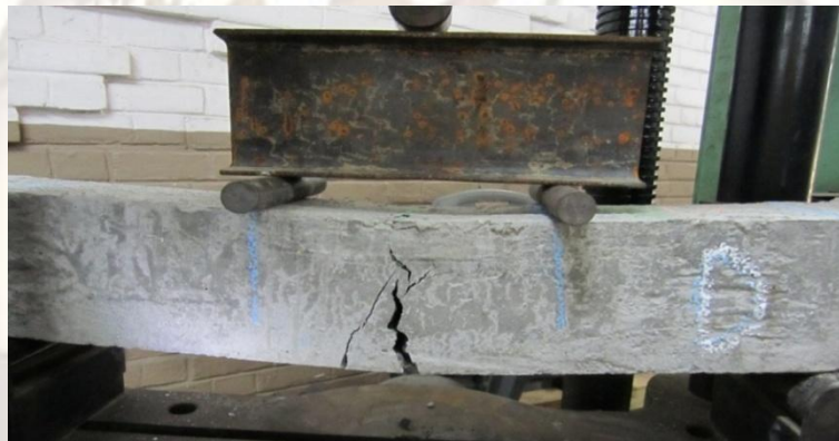
Fig.16: Failure Pattern of Doubly Reinforced Beam
