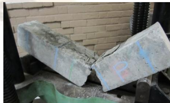
Fig.11: Cement Concrete Beam Failure
