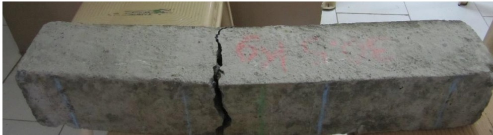
Fig.14: Failure of Singly Reinforced Beam
