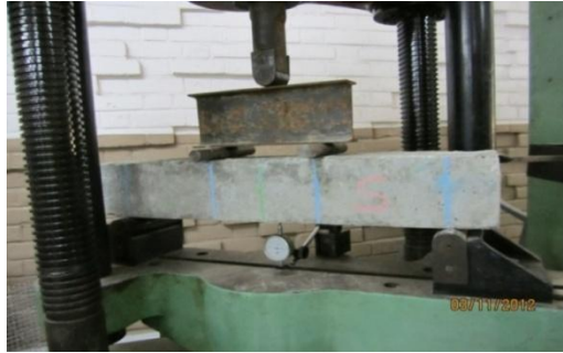
Fig.7: Test Setup to check flexural strength of Beam
