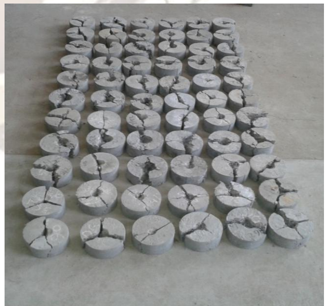
Fig No.2 Part of the specimens after ultimate failure
