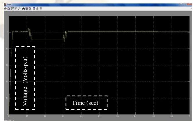
Fig.6. Voltage Sag Without DSTATCOM
