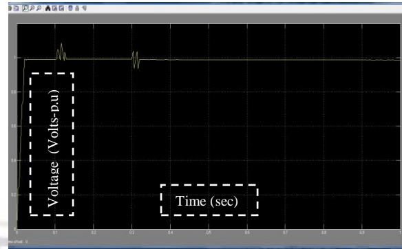
Fig.9. Voltage Swell Without DSTATCOM
