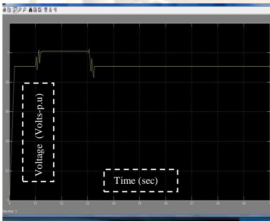
Fig.8. Voltage Swell Without DSTATCOM
