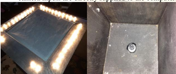
Fig. 3 Multi-touch table outside and inside view.
