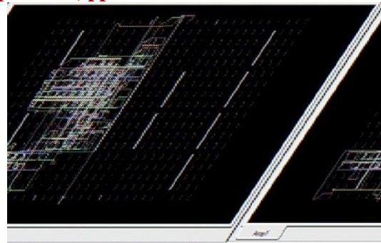
Fig 9: Routing of logical placement in targeted (xc2vpx70-7-ff1704) FPGA
