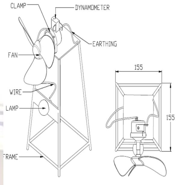
Fig 5.1 Detailed drawing of the wind energy convertor
