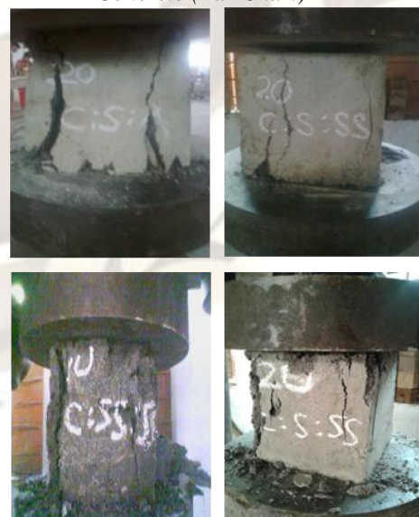
Fig 3.2 M20 Grade Concrete Compression Test
