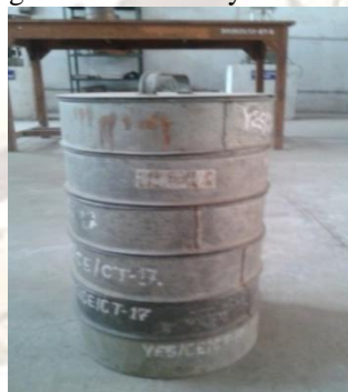
Fig.2.7 Set of Sieves for Coarse Aggregate
