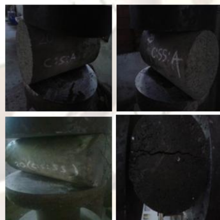
Fig.3.12 M25 Grade Split Tensile Test
