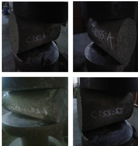
Fig 3.6 M20 Grade Split Tensile Strength (MPa)
