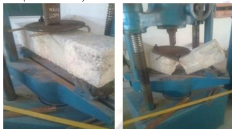
Fig.3.10 M25 Grade Concrete Flexure Test
