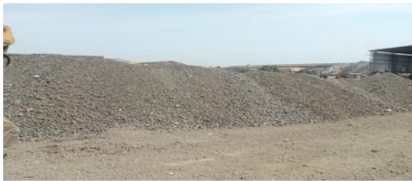
Fig.2.3 Stockpiling of steel slag aggregates at Steel Industry Wardha
