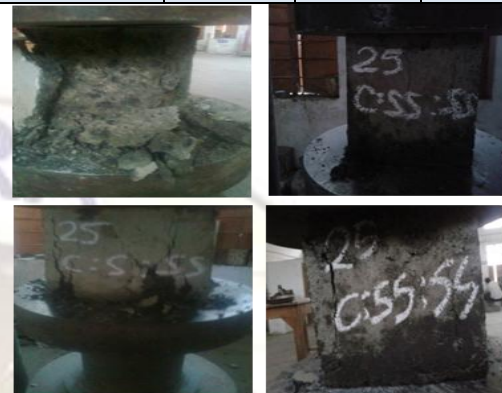
Fig.3.8 M25Grade Concrete Compression Test
