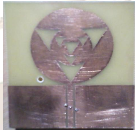
Figure 4.3 :Fabricated Circular Monopole patch Antenna.(Dark:copper,Light green:FR4 substrate)
