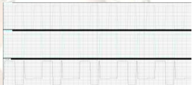
Figure9:Input and output waveform of xnor gate
