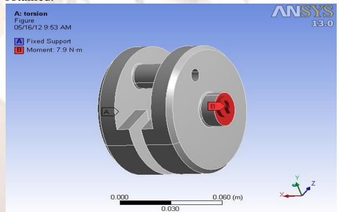
Fig.5 Torque applied at one of the journals
