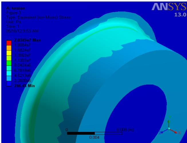
Fig.9 Maximum torsion stress in journal fillet
