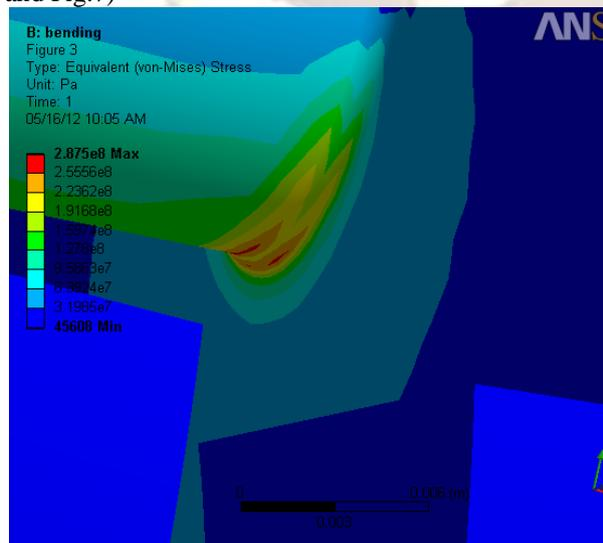
Fig.6 Maximum bending stress in crankpin fillet
