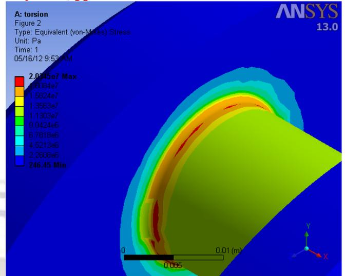
Fig.7 Maximum torsion stress in crankpin fillet
