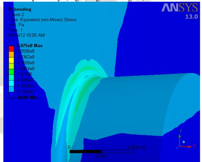
Fig.9 Maximum bending stress in journal fillet
