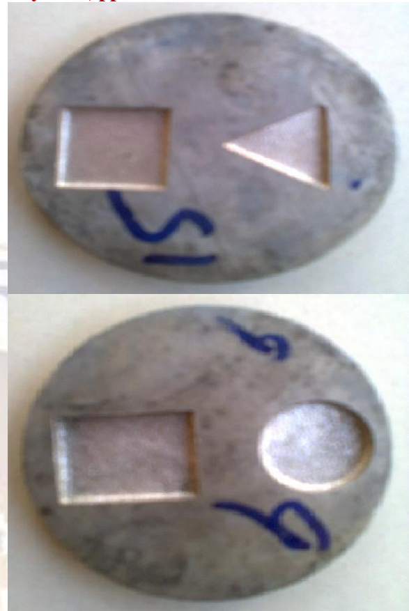
Fig. 3.1 Practically processed specimens. Fig. 3.1 shows the processed specimen of Ø 50 mm round bar of 6 mm thickness on which four geometry of tool electrode is grooved of 2 mm depth.
