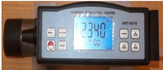
Fig 7: Photograph of Profilometer (SRT-6210).
