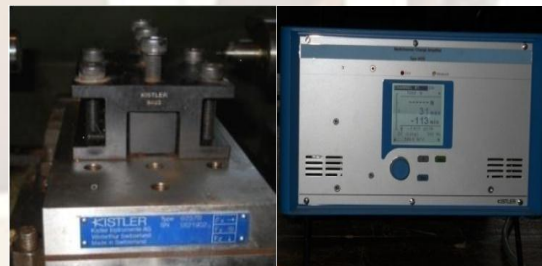
Fig. 6: Photograph of Kistler piezoelectric dynamometer and Kistler Charge amplifier
