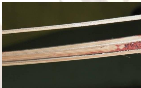
Fig4. Splitting failed specimen in tension test.
