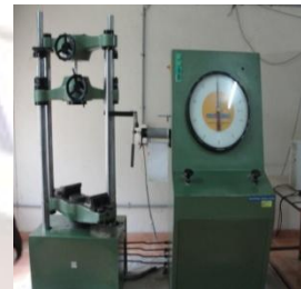
(f). Hardness test machine
