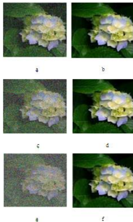
Fig. 6. (a),(b) image corrupted by 30% of salt and pepper noise and its denoised image (c),(d) image corrupted by 50% of noise and its denoised image (e),(f) image corrupted by 70% of noise and its denoised image.
