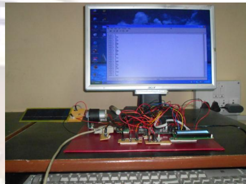
Fig. 7: Experimental setup of the proposed solar tracking system
