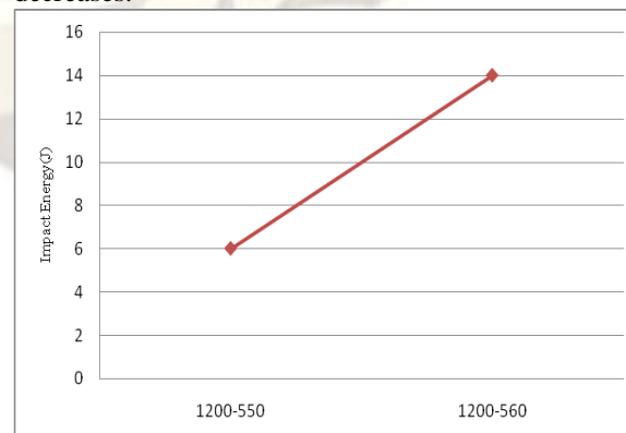
Fig. 10 Variation of impact energy against tempering temperature for different heat treatments at 1200°C hardening temperature.
