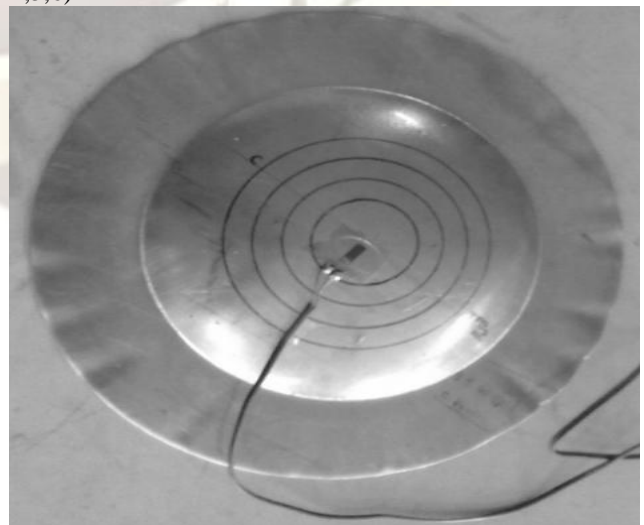
Figure 3 Bulged test specimen
