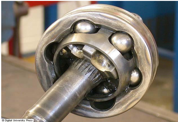
Fig. 3 Constant Velocity Joint (The type of joint more commonly used in front wheel drive cars).
