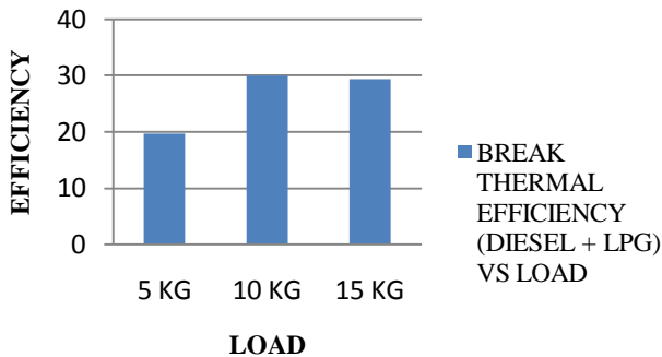
BREAK THERMAL EFFICIENCY (DIESEL + LPG) VS LOAD
