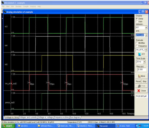
Figure 8 : output waveform of tri-state elastic buffer design
