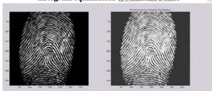
Original Image Enhanced image fig. 5 Histogram Enhancement
