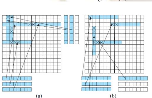
**Figure 3: The Comparison between BIRA Algorithms. (a) Repairing of the MESP, and (b) Repairing of our GESP.**
