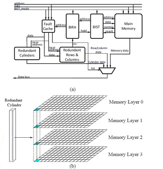
Figure 6: 3DR Architecture: (a) Modified Block Diagram, (b) Detailed Replacement Scheme
