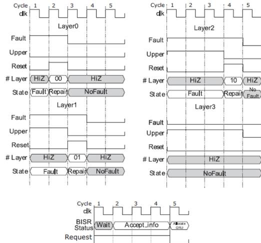
Figure 5: Timing Diagram of an Example for 3D-BISR
