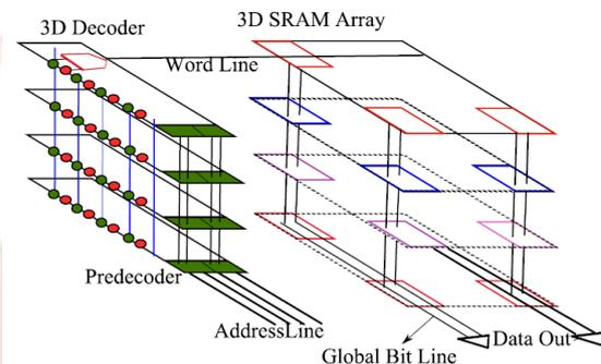
Figure 1: 3D SRAM Array Architecture
