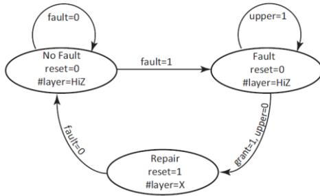
Figure 4: State Transition Diagram of the Control FSM
