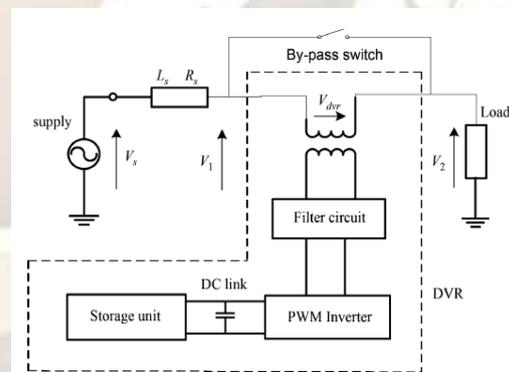
Fig. 1 Typical DVR-connected distribution system
