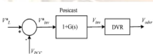
Fig. 4. Open-loop control using the Posicast controller.
