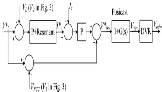
Fig.5. Multiloop control using the Posicast and P+Resonant controllers.
