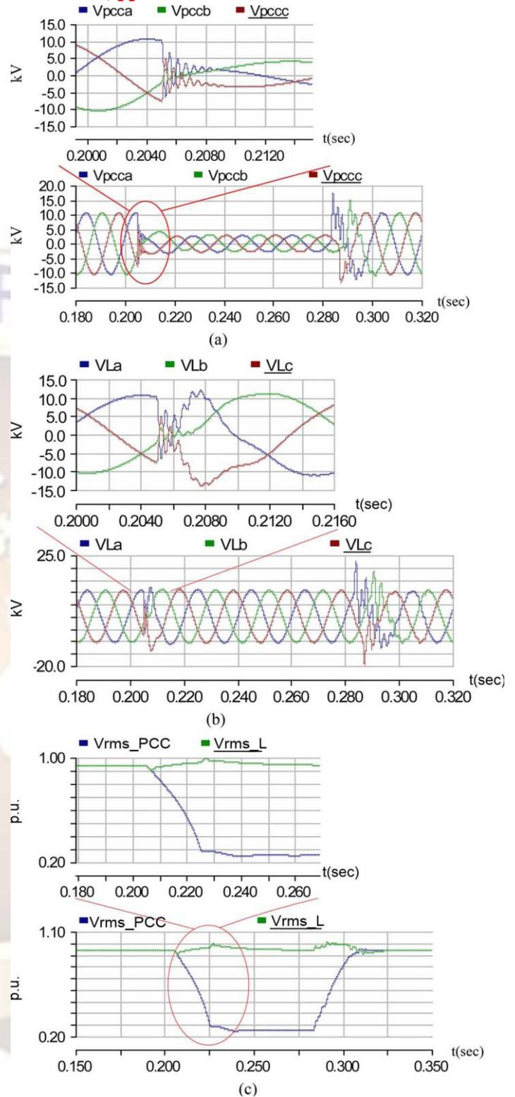
Fig. 9. Starting of an induction motor and the DVR compensation. (a) Three-phase PCC voltages. (b) Three-phase load voltages. (c) RMS voltages of PCC
