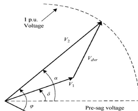
Fig. 2. Phasor diagram of the electrical conditions during voltage sag.
