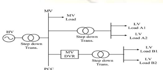
Fig. 6. DVR connected in a medium-voltage level power system.
