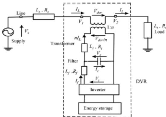
Fig.3 Distribution system with the DVR.
