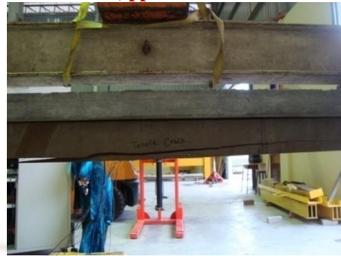
Fig. 24. Tensile crack along the timber beam at mid-span
