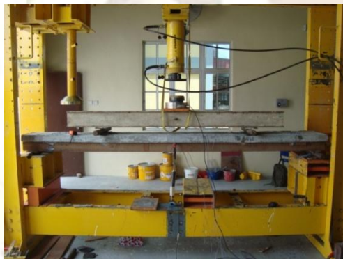
Fig. 7. The Magnus frame with the 4-connector CTC slab system specimen placed on it
