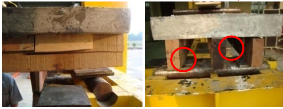
Fig. 27. Tensile crack approximately 250 mm in length along the span of 10-connector slab at the pin support: (a) Rear view; (b) Side view
