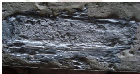
Fig. 16. Hardened composition of Sikadur-330 from plan view From the prescription manual of Sikadur-330, it takes 2 days to achieve full cure at a temperature of 35°C. The total mass of the specimens was resulted at an approximate of 220 kg each.
