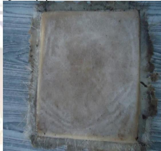
Fig. 2: composite laminate piece
