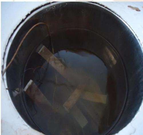
Fig.5. Constant temperature water bath with specimens
