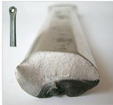
Figure 3.4.1 b) Fracture of an Aluminum Crank Arm [3]
