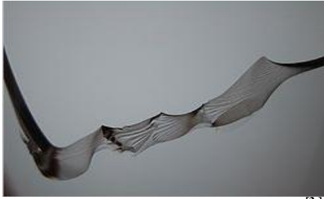
Figure 3.4.1 a) Brittle fracture in glass [3]
