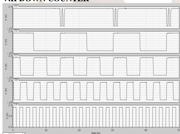
FIG. V.II Simulated Result of down counter
