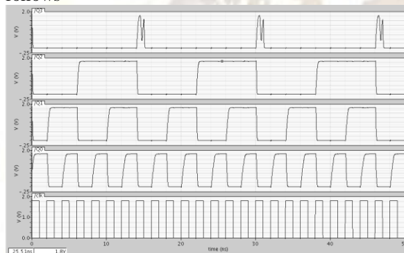
FIG. V.I Simulated Result of up counter
