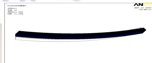
FIG.10 Total Deformation Plot for 1 st Natural Frequency
