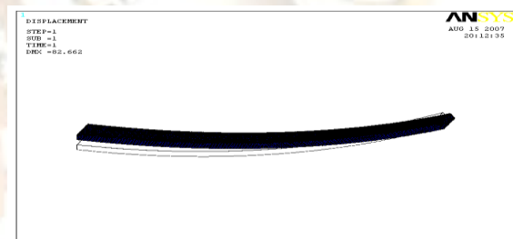
FIG.14 Deformed & Undeformed Plot of Mono Composite Leaf Spring
