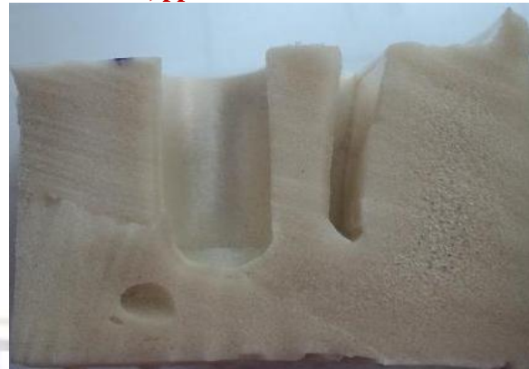
Figure 1 Non uniform microcellular structure with the use of CPW and stearic acid
