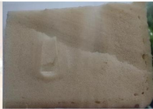
Figure 2 Uniform microcellular structure with Naphthenic oil
