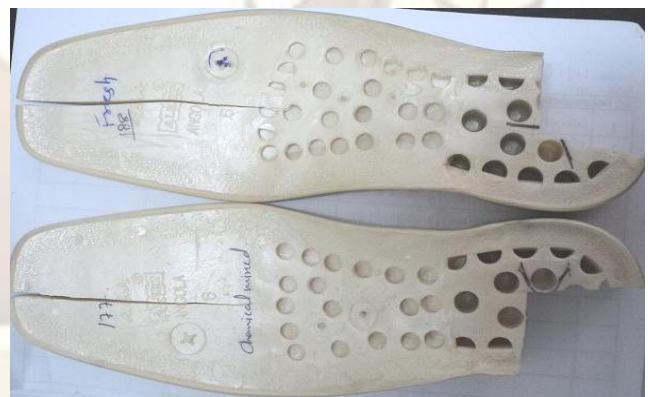
Figure 3 upper sole bright (Naphthenic oil) and lower dull bright (CPW & stearic acid)
