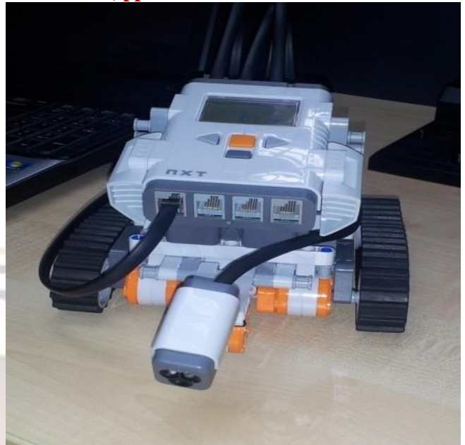
Figure 2: The Mindstorm robot with the coloured sensor attached to it to detect the flaws
