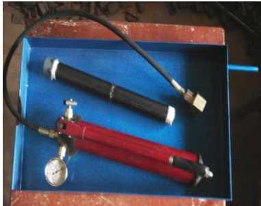
Fig. 2 Leak testing setup
